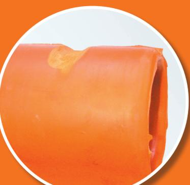
**Physical Damage:** Rope burns, deep cuts and puncture hazards are cause for rejection.
