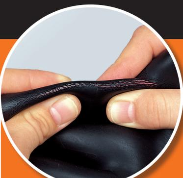
**Cracking & Cutting:**
