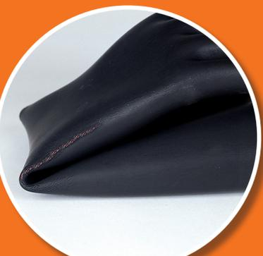
**Avoid Folding:** The strain on rubber at a folded point is equal to stretching the rubber to twice its length.
