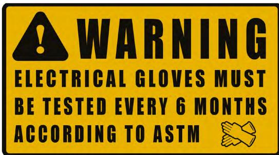
Rubber insulating gloves are the only protective gloves designed for constant contact with, and protection from, energized conductors and equipment. All of the other items are designed for protection from accidental, incidental or brush contact. Arc-rated work gloves alone offer no shock
