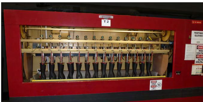
ASTM Manufacturing and Acceptance standards mandate the testing of the rubber insulating gloves by the manufacturer or supplier prior to the first delivery to the end user. Users also have the option of performing or requiring an acceptance test within
