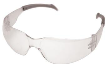
Visi-Gard® B2 Safety Glasses are made from a polycarbonate lens material that is hard-coated for scratch and impact resistance, filters more than 99% of UVA and UVB ultraviolet light and meet ANSI Z87.1+ High Impact Standards. The wraparound frame is lightweight and comfortable and offers a full panoramic view. The rubber ear tips provide a secure fit. Available in a clear frame with a clear, anti-fog lens, or a gray frame with a gray, anti-fog lens.
