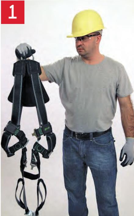
1 Hold harness by back D-ring. Shake harness to allow all straps to fall in place.
