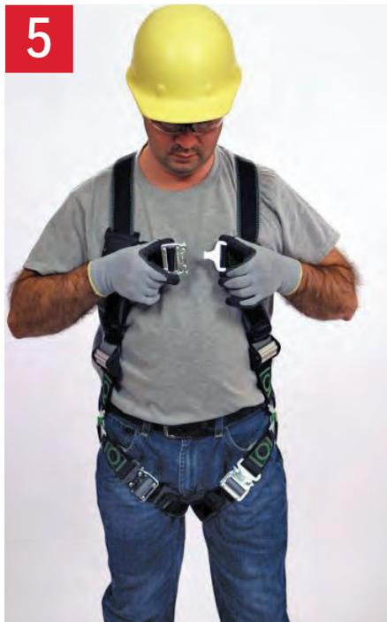
5 Connect chest strap and position in midchest area. Tighten to keep shoulder straps taut.
