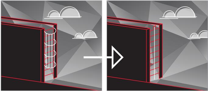
Fixed ladder cages and wells will be phased out and replaced with ladder safety systems or personal fall arrest systems.
